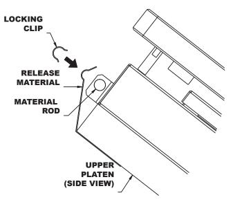
5. Check alignment and tightness of release material against upper platen.
